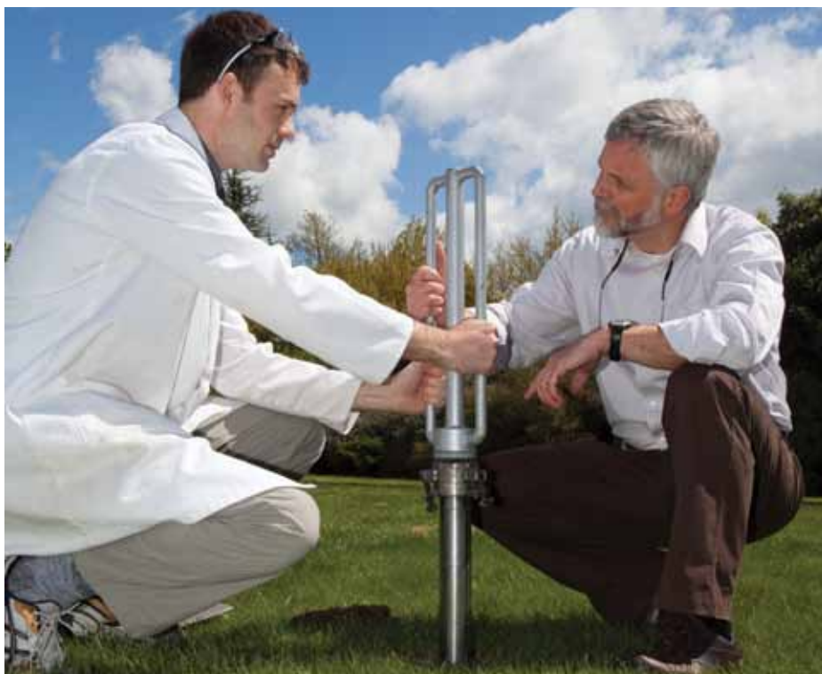
Chris Dunlop demonstrates some recent improvements in a soil coring method to measure soil carbon stocks
